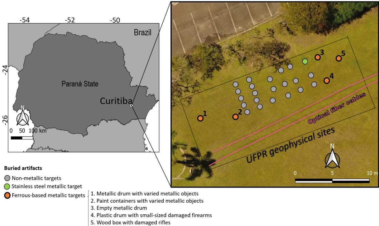
Figure 1 – Buried magnetic targets and other geophysics test sites at Polytechnic Center (UFPR), Curitiba, Paraná. Background image from <http://www.campusmap.ufpr.br>.
